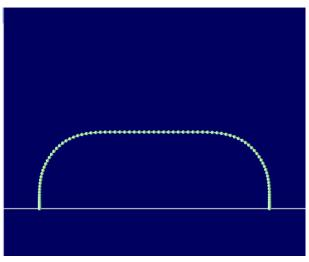
MOVEPICK is basically an absolute move to a position in 3..6 axes. However the motion includes an incremental "withdraw" amount and special controls for the move speed profile to allow fast pick
