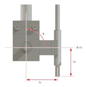
The direction of motion on all 5 axes MUST match the diagram for the FRAME 16 transformation to operate. If an axis direction of motion is inverted it can be reversed either:
