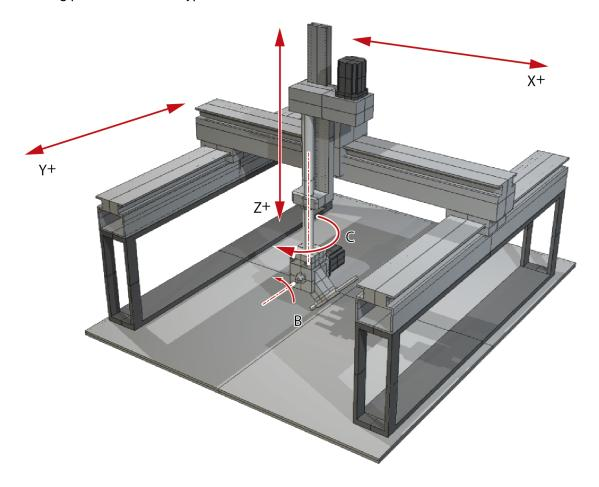
Once the frame is enabled DPOS on the X, Y and Z axis are measured in axis counts. The wrist axis is set to use Nanoradians. You can of course set UNITS for all axis to any suitable scale.
