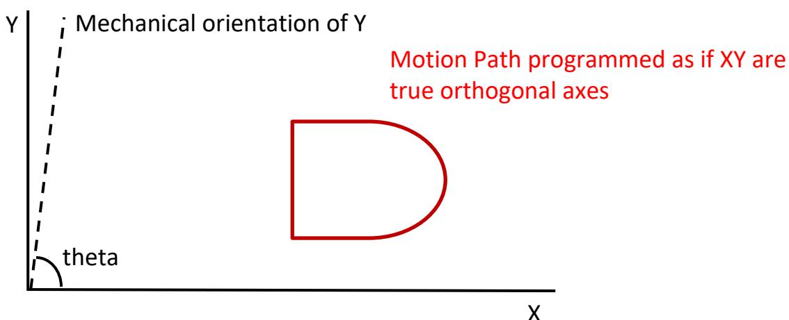
Compensation for miss-aligned Y axis orientation. Angle in Radians.
