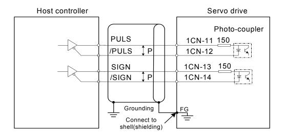
Example 2 (When host device is open collector output subject to 24VDC signal power)
