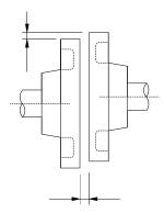
Measure this at four quarter positions of a cycle. The difference between the maximum and minimum measured value must be less than 0.03mm. (Rotate together with shaft connectors) **Note:**
