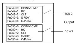
The following table shows the pin number definition for Pn049 (correspond to pin 1CN-2 output) , Pn050 (correspond to pin 1CN-3 output) .
