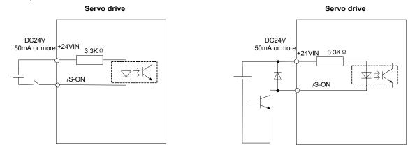
If the relay contact input is used, the relay must be suitable for low electric current, otherwise it causes signal receiving faults.
