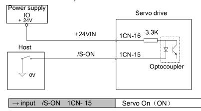
Switch servomotor between Power on and Power of, when low level is active.
