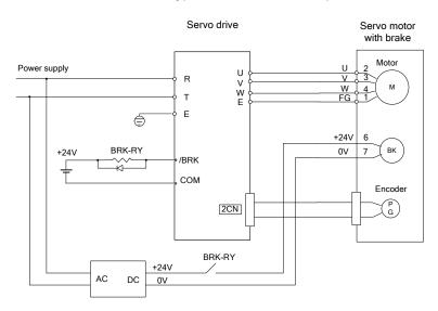
BRK-RY: brake sticking control relay
