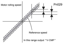
With the user's constant as below, the range of output /V-CMP can be designated.
