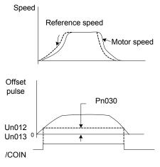
Un012:error pulse counter low position monitoring Un013:error pulse counter high position monitoring When output is active at low level:
