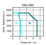
(A: Continuous working area, B: Repeatable working area)
