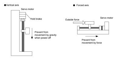
Make sure servomotor is mechanically separated before confirming action of servomotor and brake active (holding brake) . If all the parts are moving well, connect servo motor to the machine.
