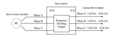
Divides pulse frequency of servomotor encoder(PG) and output according to pulse number setting.
