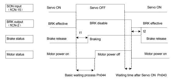
t1,t2:determined by external relay and brake loop move time
