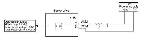
External +24V I/O power supply is required, since there is no +24V power supply available inside servo drive.
