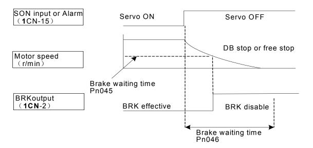
For running a brake motor, if S-OFF is caused by variation of /S-ON or alarm occurrence, it's required to set brake waiting speed of servomotor or brake waiting time.
