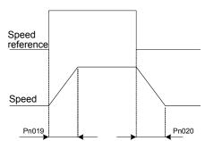
Inside servo drive, perform acceleration and deceleration of the set value on speed reference to implement speed control.
