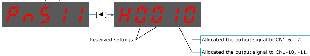
Figure 5-3 Output signals allocated
