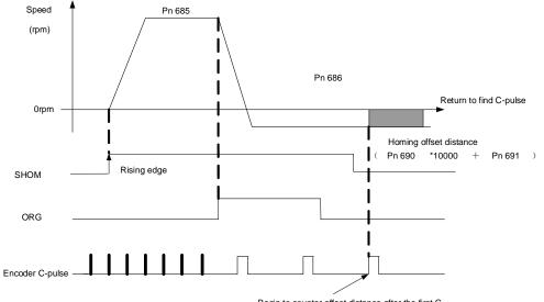
Begin to counter offset distance after the first Cpulse is produced when leaving zero posiion.
