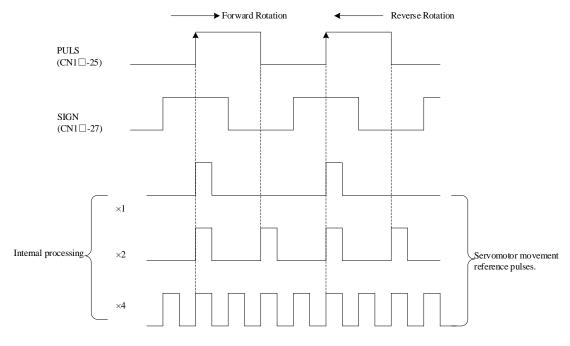
The input pulse multiplier can be set for the two-phase pulse train with 90° phase differential reference pulse form.
