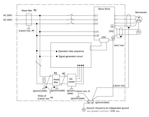
When using a noise filter, always observe the following wiring instructions:
