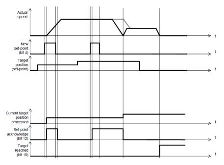
When the speed profile is S (motion\_profile\_type=2), only set of setpoints is available. 6083 h (profile\_acceleration) limits max. acceleration. 6081h (profile\_velocity) limits max.speed. 60A4-01 h (VAR Profile\_jerk1) limits the jerk.now only symmetrical S linear is available.
