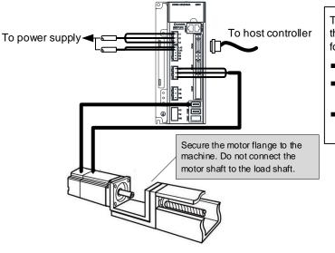
The servomotor is operated without connecting the shaft to the machine in order to confirm the following wiring is correct.
