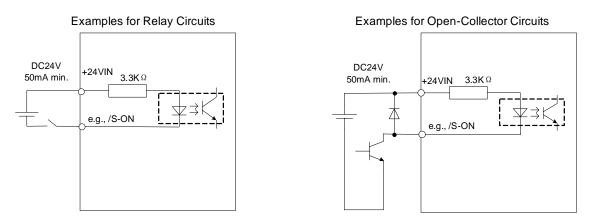
Select a low-current relay for the relay circuits, or a faulty contact may be caused.
