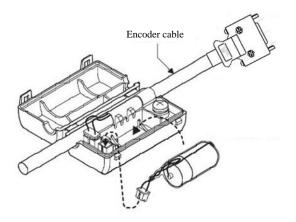
Step 3 Cover the shell of the battery case.
