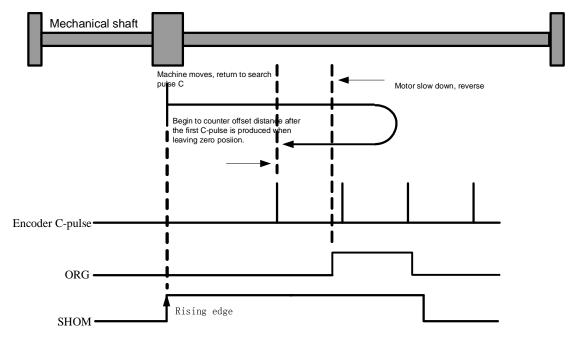
After hitting the origin signal ORG, the motor will find C-pulse directly; the figure is shown as below:
