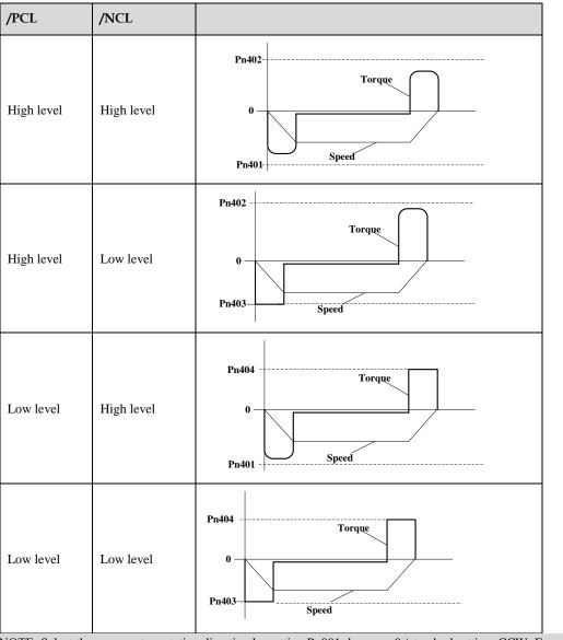
NOTE: Select the servomotor rotation direction by setting Pn001=b - - 0 (standard setting, CCW=Forward direction).
