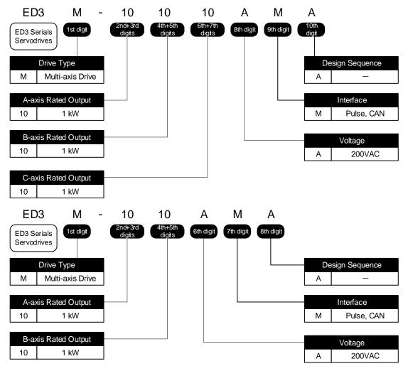
[NOTE] All the axis of ED3M servodrive controlled can be applied for the motor power of 50W to 1kW, those also can be set up to treble in overload capability.
