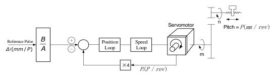
In which,  $\Delta \ell$  is reference unit;  $P_G$  is encoder pulse; P is ball screw pitch;  $\frac{m}{n}$  is deceleration ratio.
