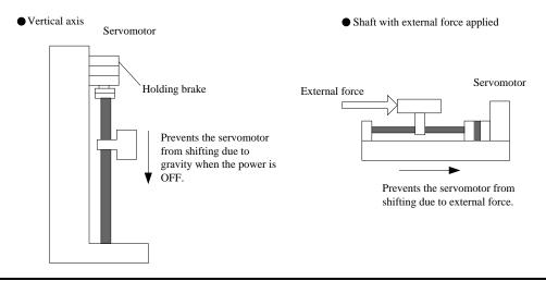
• The servomotor with the built in brake, is a de-energization brake. It is used to hold the servomotor and cannot be used as a braking purposes. Use the holding brake only to hold a stopped servomotor.
