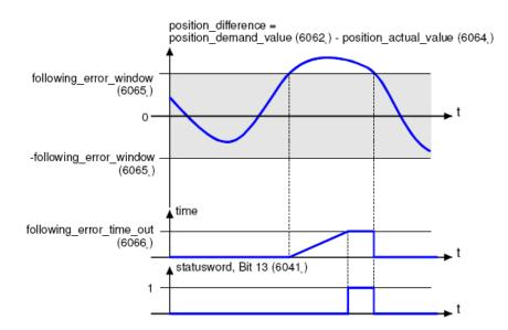
The deviation of the actual position value (**position\_actual\_value**) from the desired position value (**position\_demand\_value**) is named trailing error. If for a certain period of time this trailing error is bigger than specified in the trailing error window (**following\_error\_window**) bit 13 (**following\_error**) of the object **statusword** will be set to 1.
