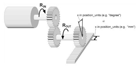
To calculate the **position factor** the following values are necessary:
