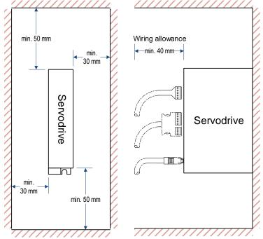
• When you install more than one Servodrive in the control panel, provide the following intervals between the Servodrives and spaces around the Servodrives. Install cooling fans above the Servodrives so that hot spots do not occur around the Servodrives.
