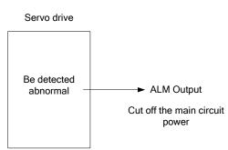
Normally, the external circuit consists of /ALM should be able to switch off the power of servo drive.
