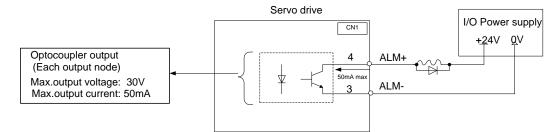
An external +24V I/O power supply is required since there is no +24V power source available inside the servo drive.
