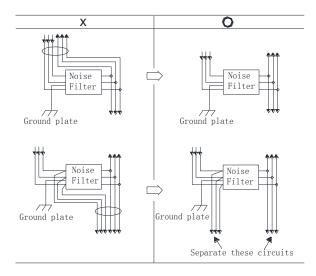
• Separate the noise filter ground wire from the output lines. Do not accommodate the noise filter ground wire, output lines and other signal lines in the same duct or bundle them together.
