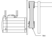
Adjust the belt tension to adjust the radial load. Measure the belt tension at 45° intervals of the machine shaft. Turn the shaft and take measurements with a belt tension meter at each point.
