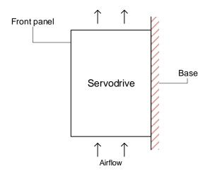
A fan can be added to force cooling the Servodrive if necessary.
