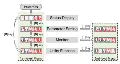
Note: Only under the 1st-level menu, press the [AXIS] key to switch the control among axis-A, axis-B and axis-C.
