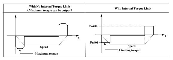
NOTE: Too small a torque limit setting will result in insufficient torque during acceleration and deceleration.
